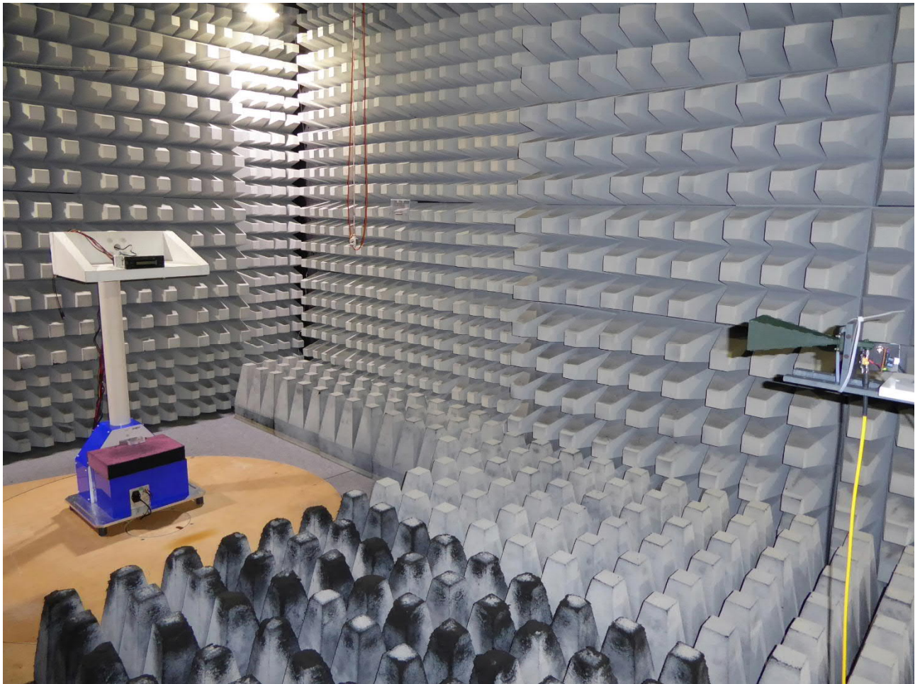
Test setup fully anechoic chamber (12 - 18 GHz)
