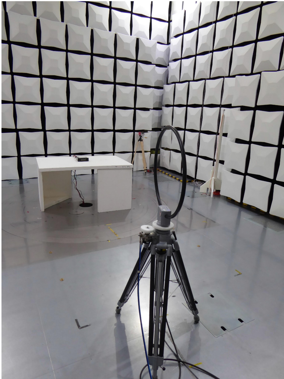
Test setup semi anechoic chamber (9 kHz – 30 MHz) – Pos 2
