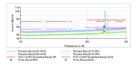
The peaks above the limit are BT EDR Chipset #1, WLAN 2.4 GHz Chipset #1 and BT EDR Chipset #2 carriers.
