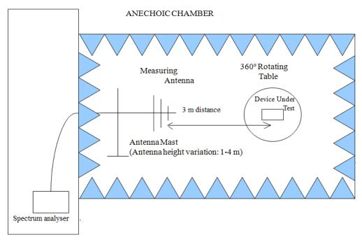
Shielded Control Room For Radiated Measurements
