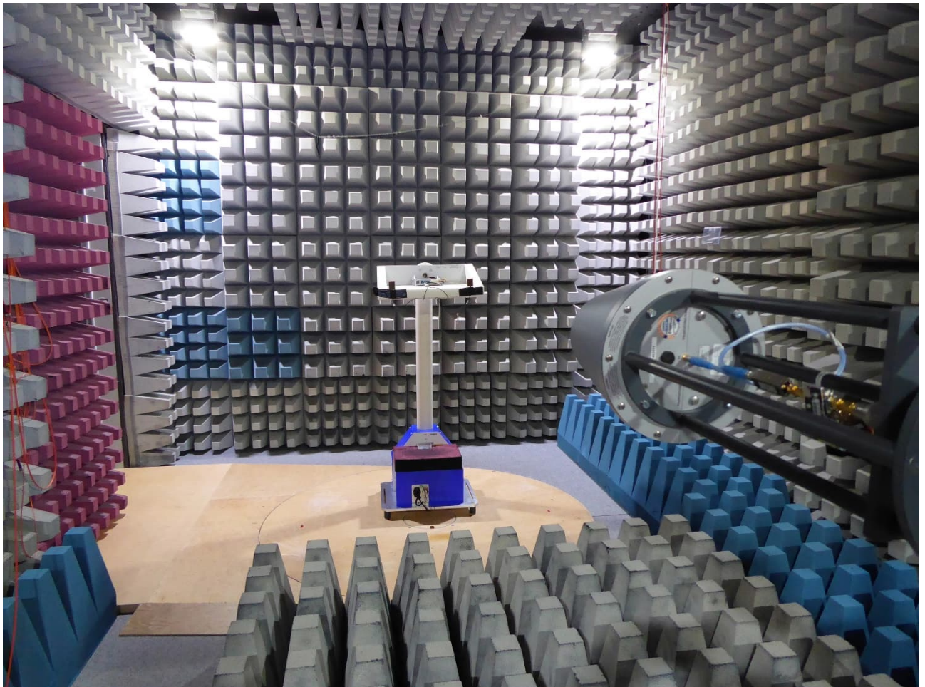
Test setup fully anechoic chamber (1 - 8 GHz)
