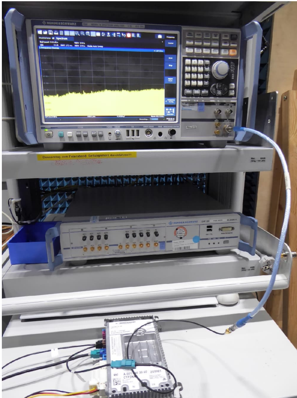
Test setup antenna port conducted – connector BT/WiFi 2
