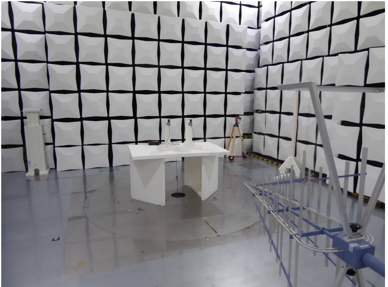
Test setup semi anechoic chamber (30 MHz – 1 GHz)
