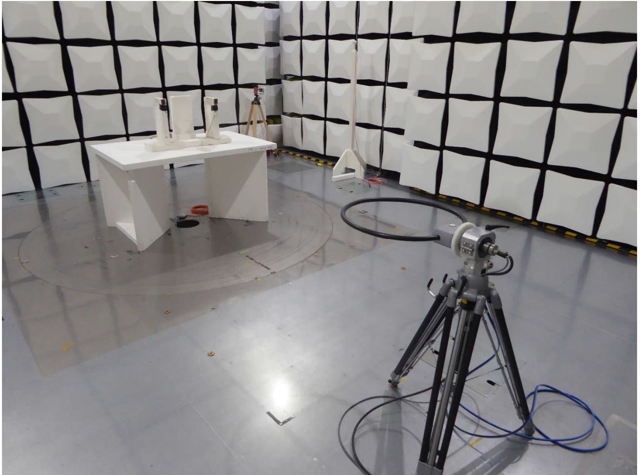
Test setup semi anechoic chamber (9 kHz – 30 MHz) – Meas Ant pos. 3
