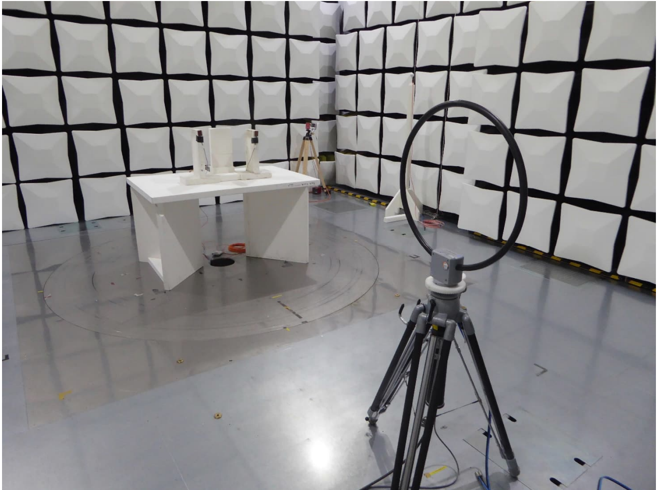
Test setup semi anechoic chamber (9 kHz – 30 MHz) – Meas Ant pos. 2
