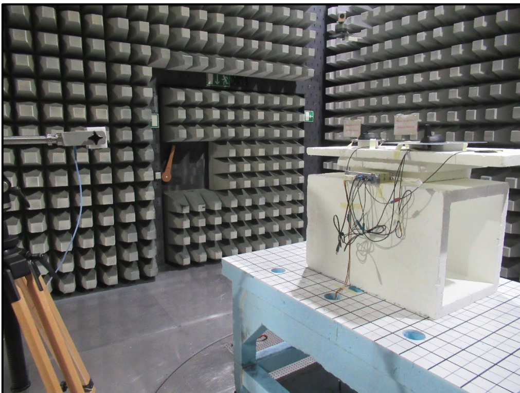
Photo 8 Radiated Test Setup from 18 GHz to 40 GHz
