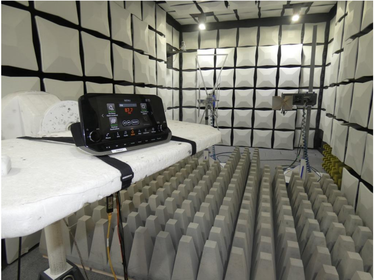
Photo 5: Test setup for radiated measurements (1 GHz – 26 GHz; FCC 15c247)
