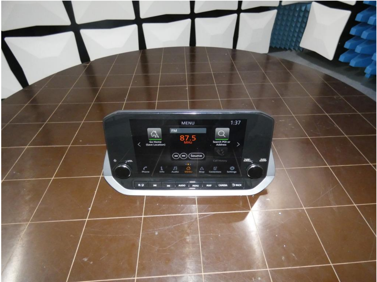
Photo 6: Test setup for radiated measurements, front view
