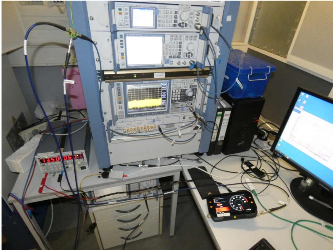
Photo 2: Setup for conducted measurements at temporary antenna ports
