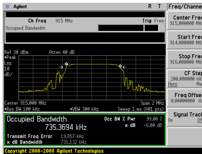
99%OBW&6dB Bandwidth plot on channel 13
