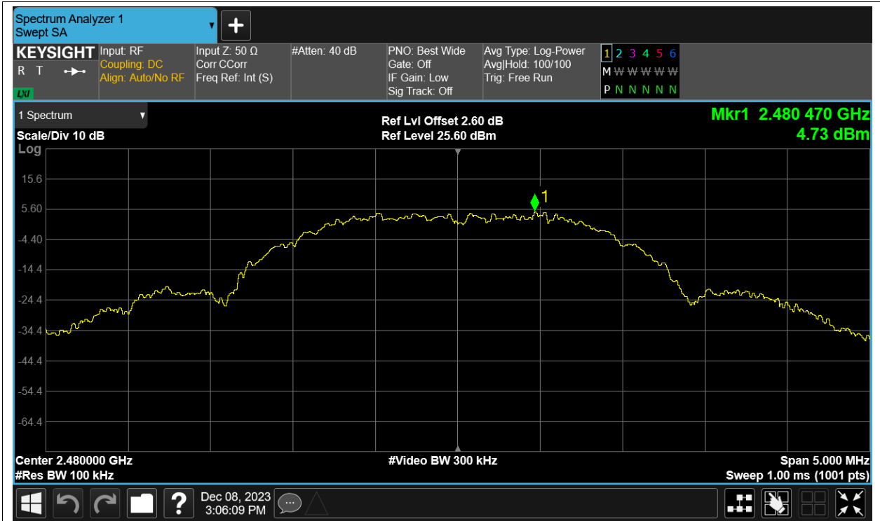
Tx. Spurious NVNT ZigBEE 2480MHz Ant1 Emission
