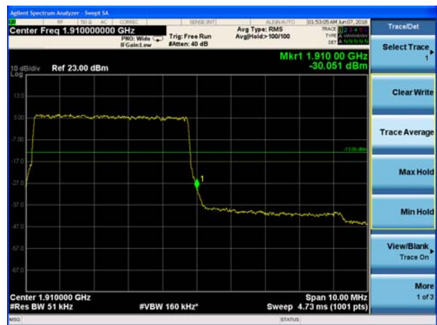
LTE Band 2 5MHz QPSK 100%RB CH-High
