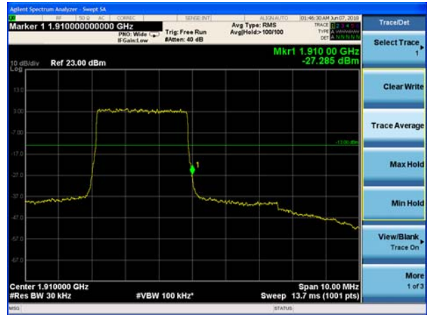
LTE Band 2 5MHz QPSK 1RB CH-High
