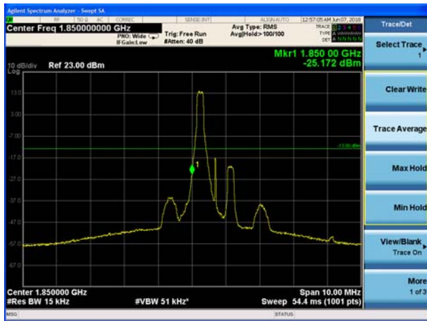
LTE Band 2 1.4MHz QPSK 100%RB CH-Low
