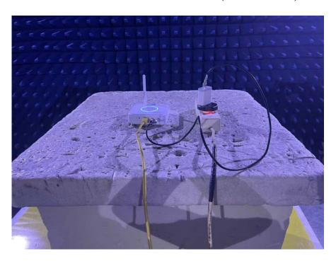
Radiated Emissions - Rear View (Above 1GHz)
