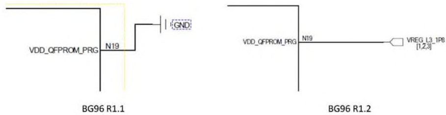
Figure 1: Schematic Designs of BG96 R1.1 and R1.2
