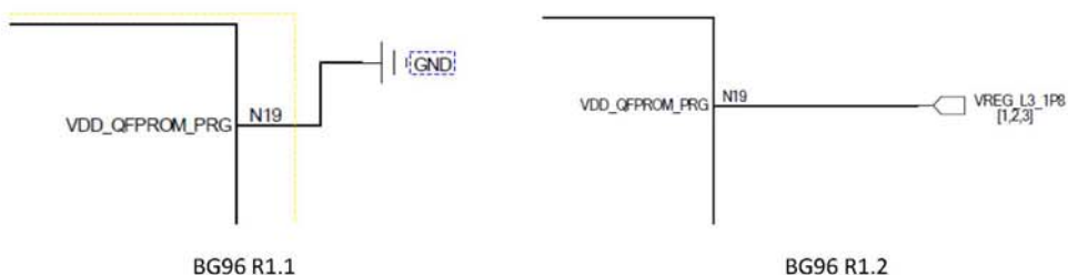
Figure 1: Schematic Designs of BG96 R1.1 and R1.2
