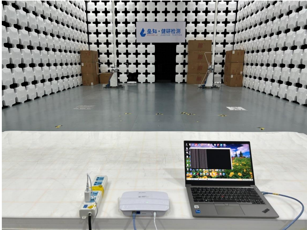
Radiated Spurious Emission Below 1GHz
