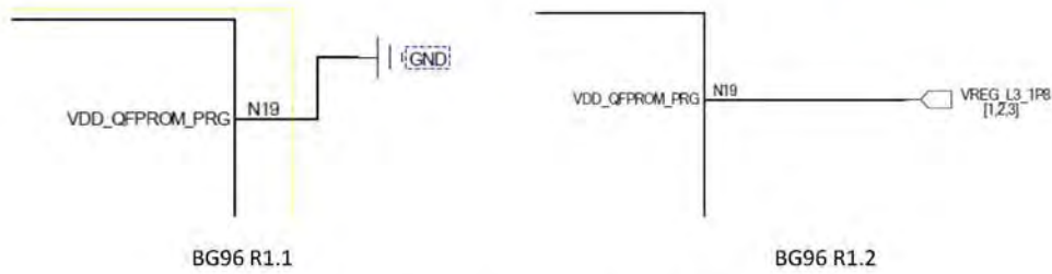
Figure 1: Schematic Designs of BG96 R1.1 and R1.2
