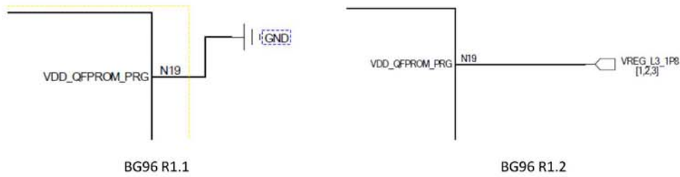
Figure 1: Schematic Designs of BG96 R1.1 and R1.2
