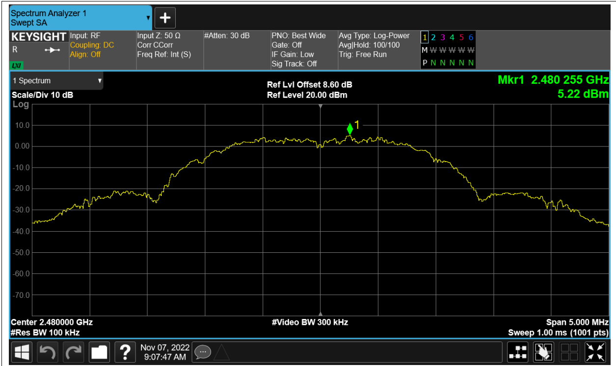
Tx. Spurious NVNT ZIGBEE 2480MHz Ant1 Emission
