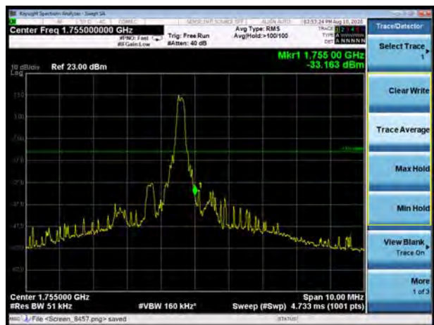
LTE Band 4 QPSK 3MHz CH-High, 1 RB
