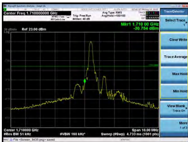
LTE Band 4 16QAM 3MHz CH-Low, 1 RB
