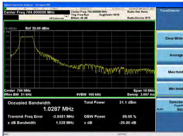
LTE Band 12 16QAM 10MHz CH-Middle
