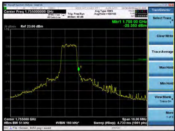
LTE Band 4 QPSK 3MHz CH-High, 1 RB
