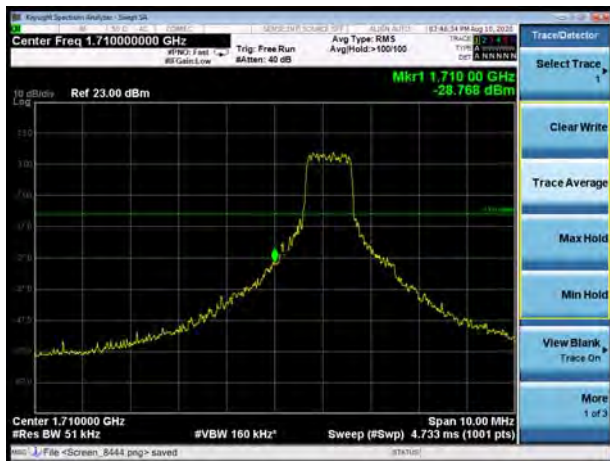
LTE Band 4 16QAM 15MHz CH-Low, 1 RB
