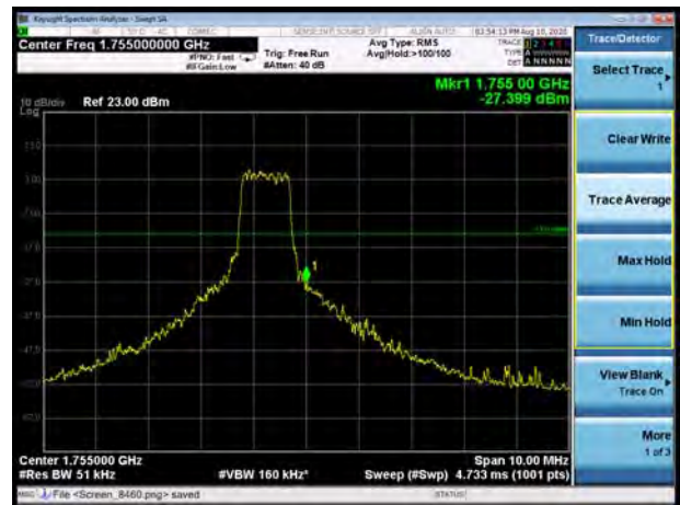
LTE Band 4 16QAM 5MHz CH-High, 1 RB
