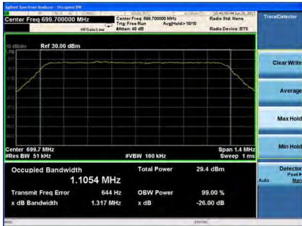
LTE Band 12 QPSK 1.4MHz CH-Middle
