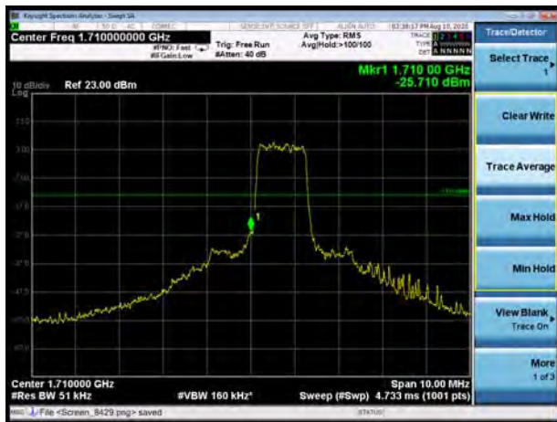
LTE Band 4 QPSK 3MHz CH-Low, 1 RB
