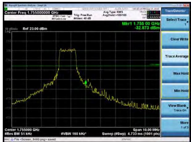
LTE Band 4 QPSK 15MHz CH-High, 1 RB
