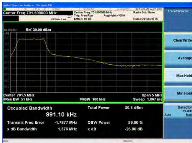
LTE Band 12 16QAM 5MHz CH-Middle
