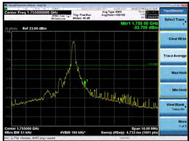
LTE Band 4 16QAM 10MHz CH-High, 100%RB
