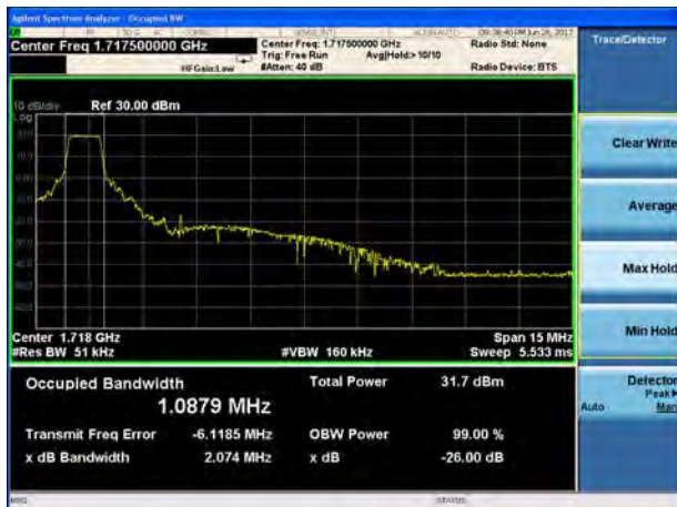
LTE Band 4 16QAM 15MHz CH-Middle
