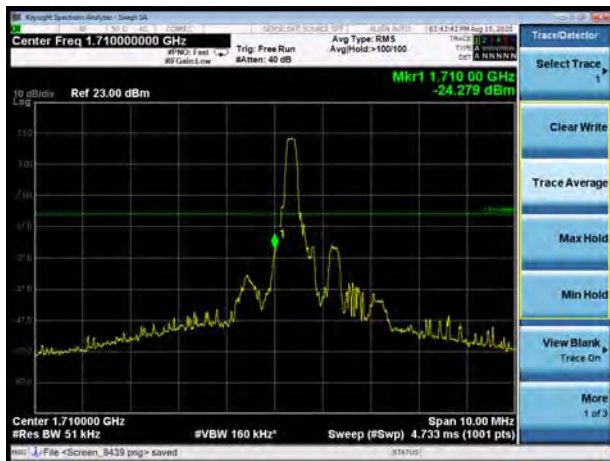
LTE Band 4 16QAM 5MHz CH-Low, 100%RB
