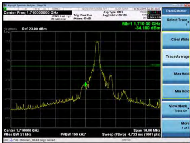
LTE Band 4 16QAM 10MHz CH-Low, 100%RB
