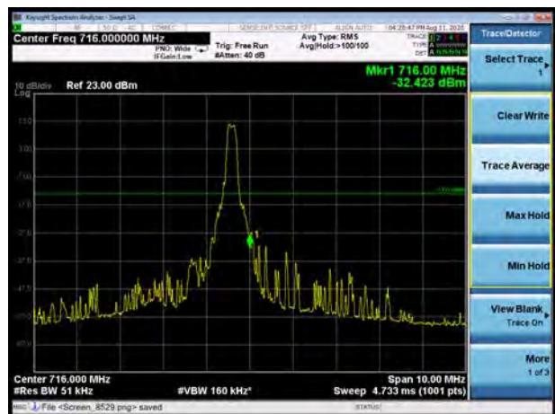
LTE Band 12 QPSK 3MHz CH-High, 1 RB
