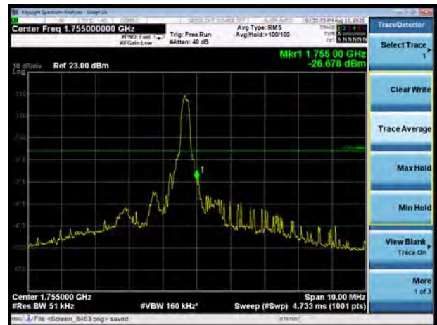
LTE Band 4 16QAM 5MHz CH-High, 100%RB
