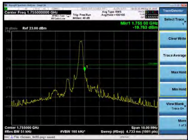
LTE Band 4 16QAM 1.4MHz CH-High, 100%RB
