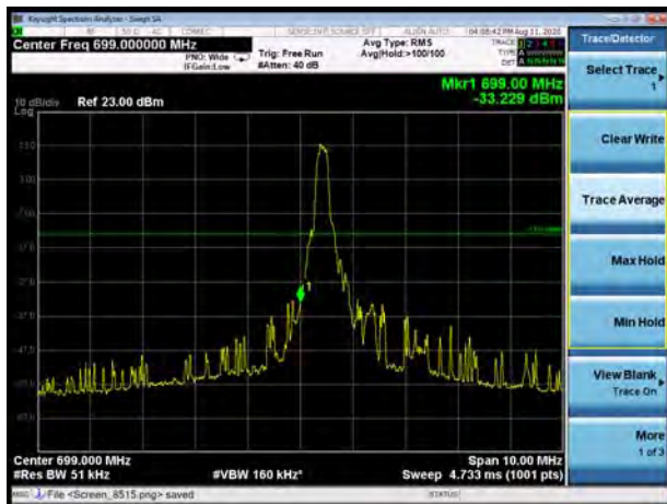
LTE Band 12 16QAM 3MHz CH-Low, 100%RB
