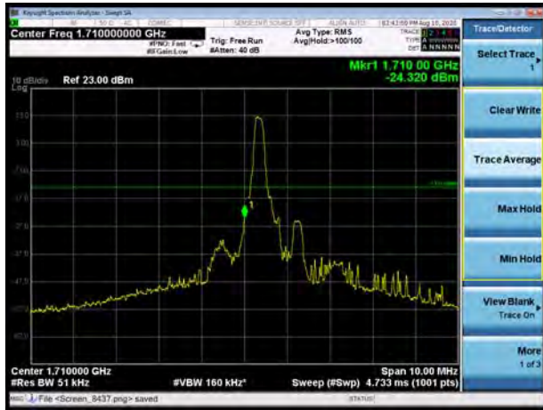
LTE Band 4 QPSK 5MHz CH-Low, 100%RB
