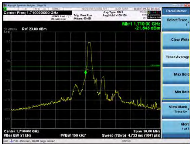
LTE Band 4 16QAM 1.4MHz CH-Low, 100%RB
