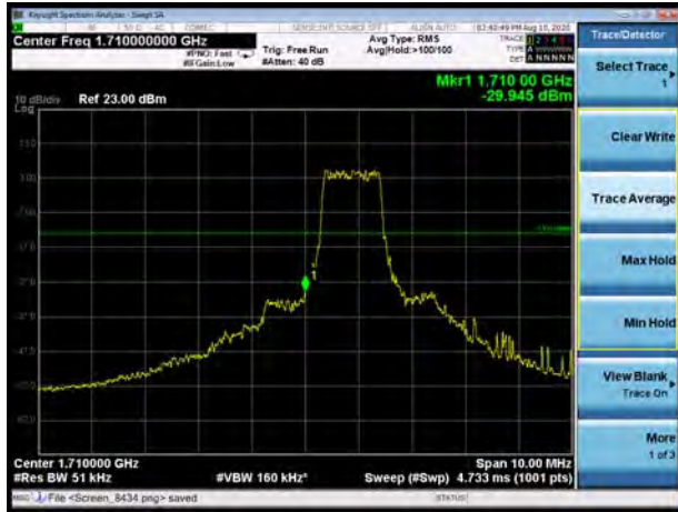
LTE Band 4 QPSK 5MHz CH-Low, 1 RB
