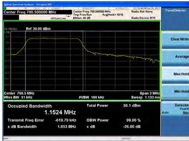
LTE Band 12 QPSK 3MHz CH-Middle
