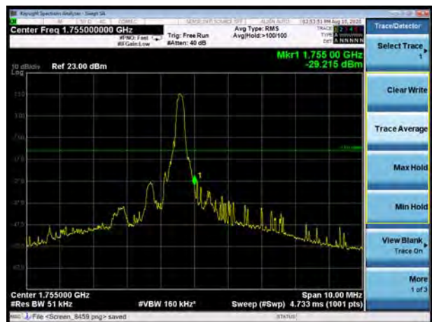
LTE Band 4 16QAM 3MHz CH-High, 1 RB
