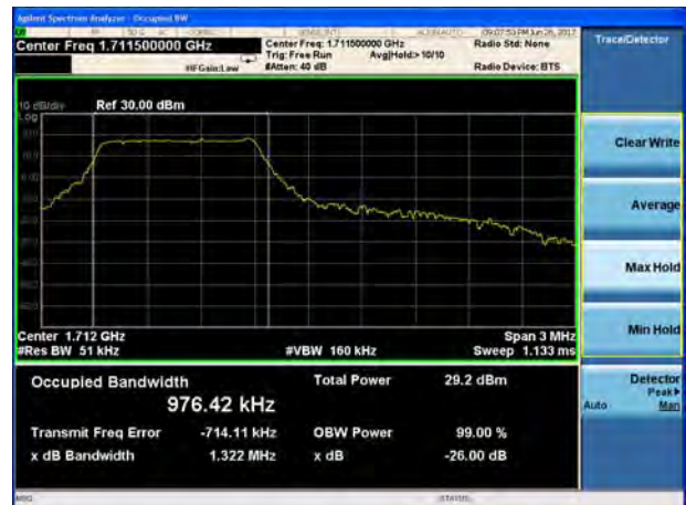
LTE Band 4 16QAM 3MHz CH-Middle
