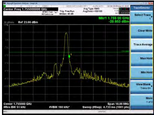
LTE Band 4 QPSK 1.4MHz CH-High, 100%RB
