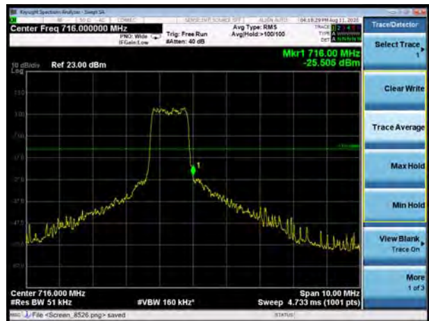
LTE Band 12 QPSK 3MHz CH-High, 1 RB
