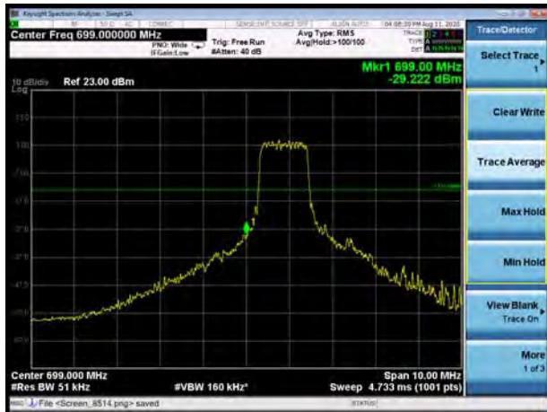
LTE Band 12 QPSK 5MHz CH-Low, 1 RB
