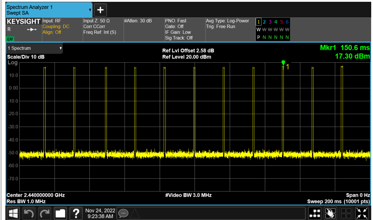
Duty Cycle NVNT user 2480MHz Ant1
