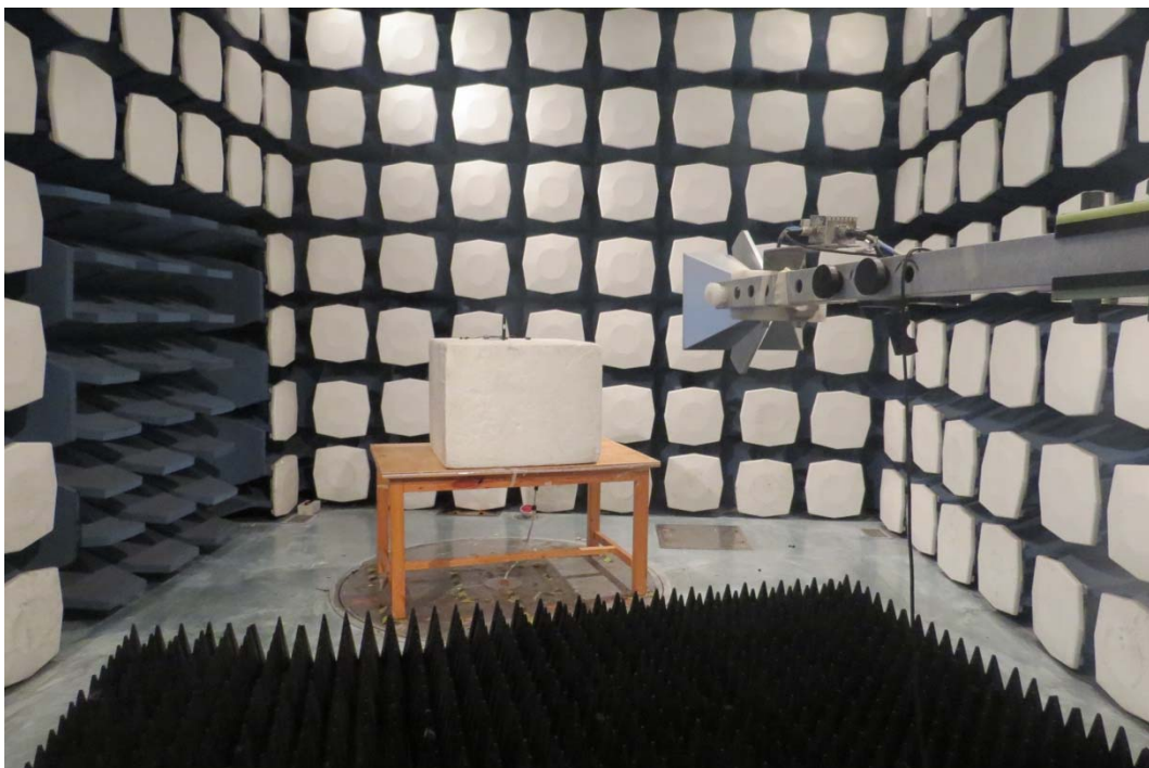
Picture 2: Radiated Spurious Emissions Test setup
