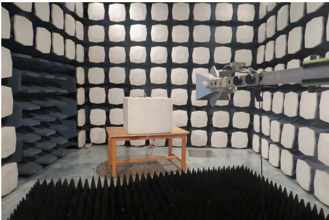
Picture 2: Radiated Spurious Emissions Test setup
