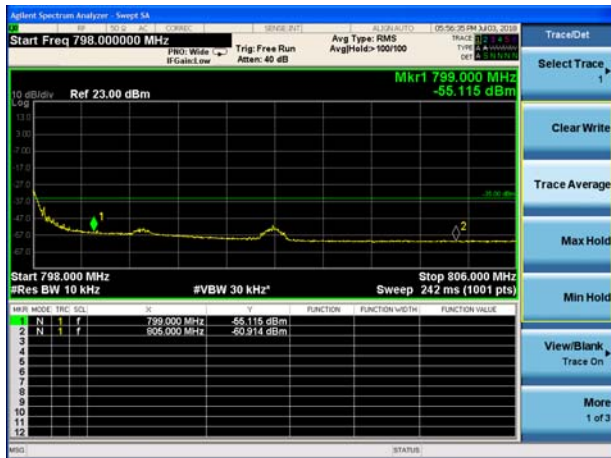
LTE Band 14 QPSK 5MHz 1 RB (799MHz ~805MHz)
