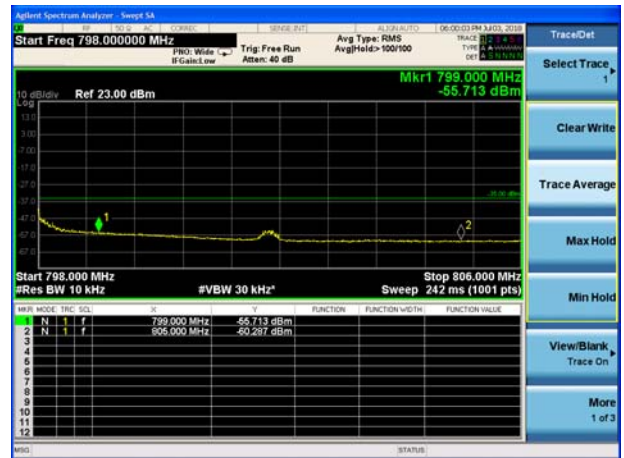
LTE Band 14 QPSK 10MHz 1 RB (799MHz ~805MHz)
