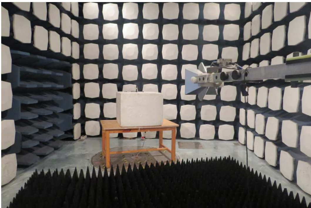
Picture 2: Radiated Spurious Emissions Test setup
