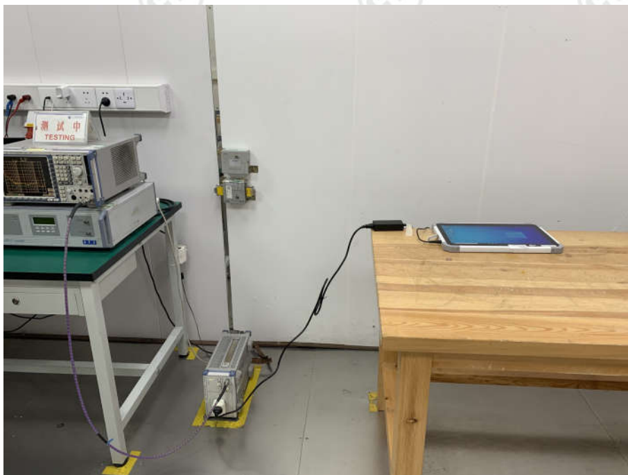
Conducted Emissions Test Setup
