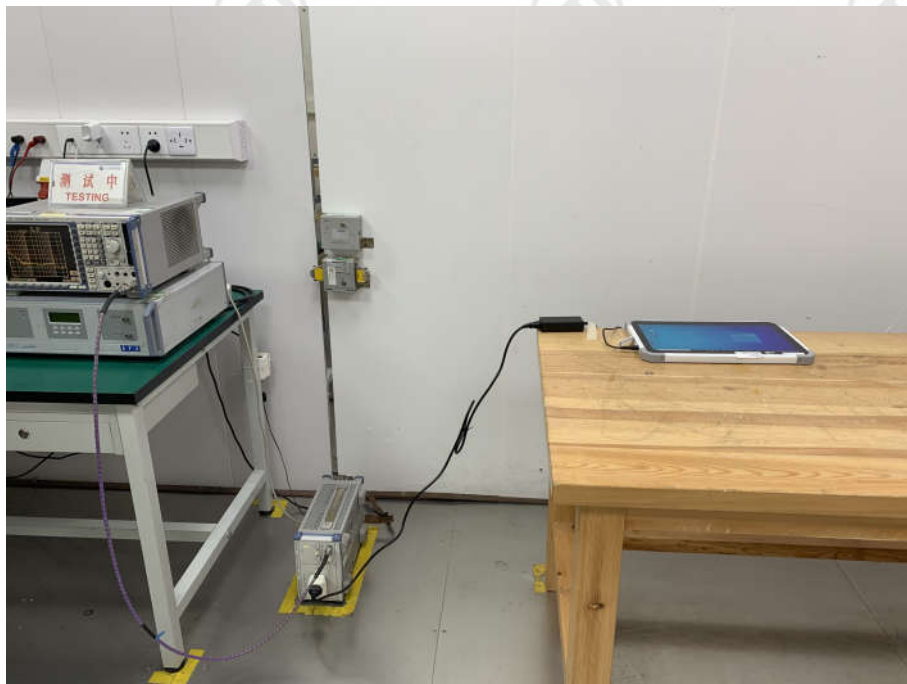
Conducted Emissions Test Setup
