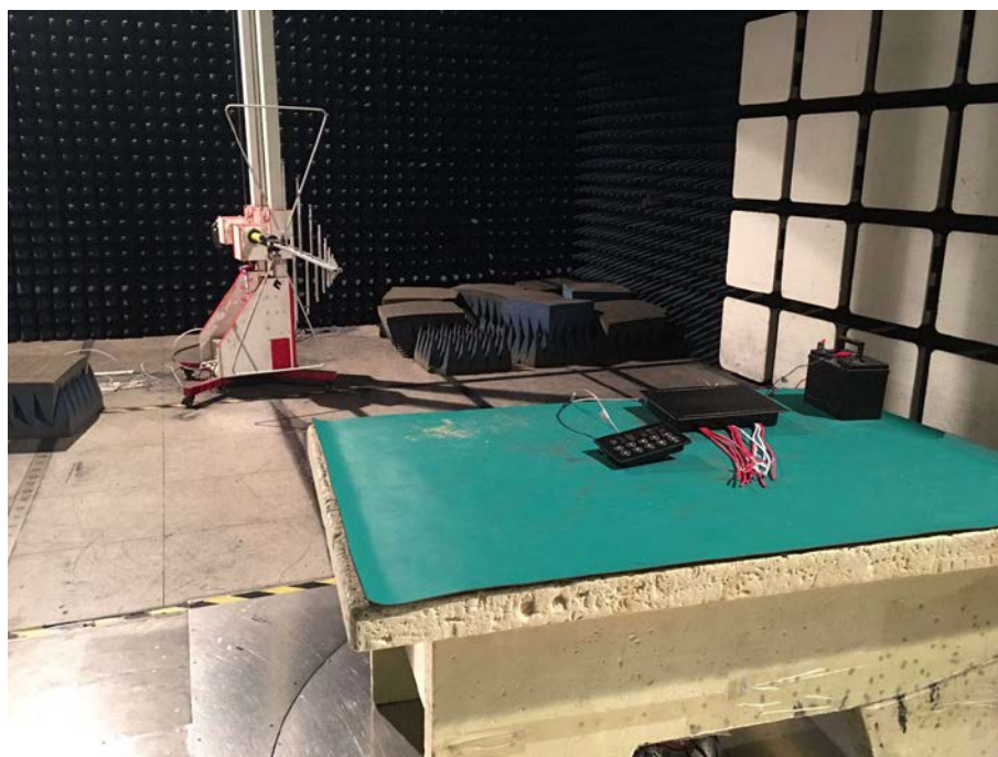
Spurious Emission Test Setup (Above 1GHz)
