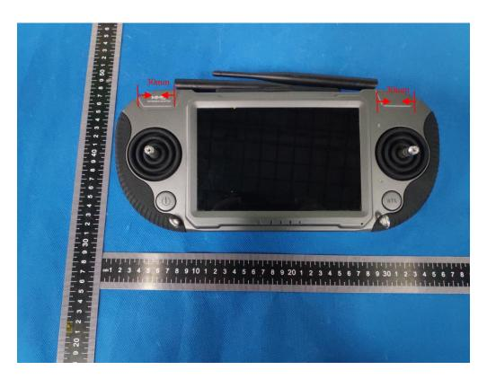
Note: The distance between the antenna and the human finger during actual use is 30mm. **Conclusion:**
