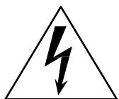
This lightning flash symbol is intended to alert the user to the presence of uninsulated and “dangerous voltage” within the mixer's enclosure that may be of sufficient power to constitute a risk of electric shock.
