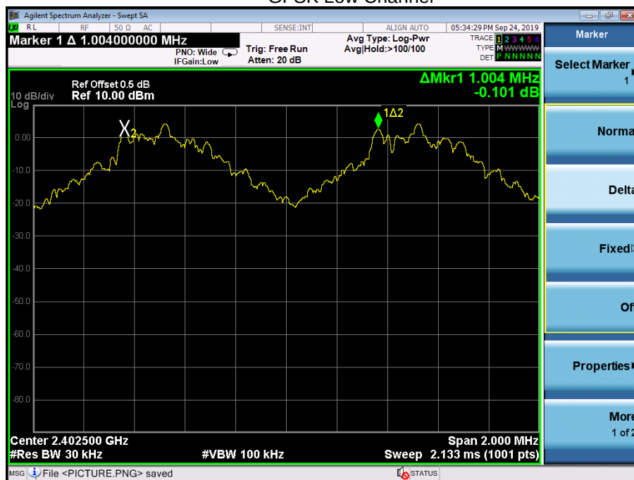
Test plots GFSK Low Channel
