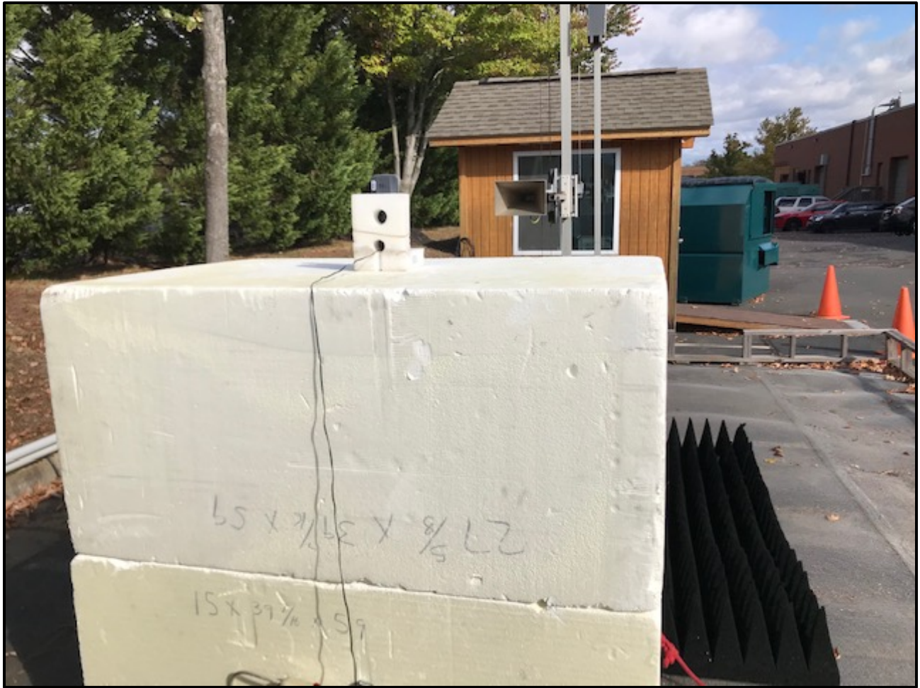
Photograph 4: Radiated Emissions Testing – Back View (Spurious Emissions, >1 GHz)
