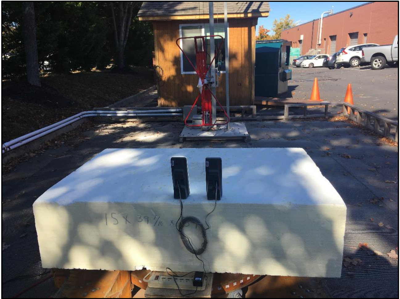
Photograph 2: Radiated Emissions Testing – Back View (Digital Emissions, <1 GHz)
