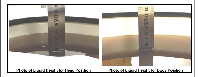
The dielectric properties of the head tissue simulating liquids are defined in IEEE 1528, and KDB 865664 D01 Appendix A. For the body tissue simulating liquids, the dielectric properties are defined in KDB 865664 D01 Appendix A. The dielectric properties of the tissue simulating liquids were verified prior to the SAR evaluation using a dielectric assessment kit and a network analyzer.
