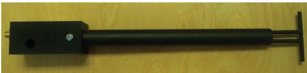
Figure 1 – MVG COMOSAR Validation Dipole
