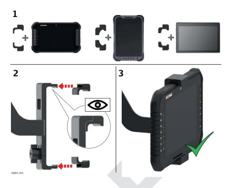
$\hfill \Box$  Attach the correct rubber to the ZHR07 holder before use.
