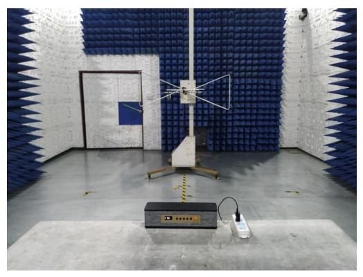
RADIATED EMISSION TEST SETUP ABOVE 1GHz
