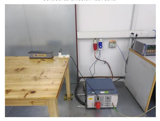
CONDUCTED TEST SETUP
