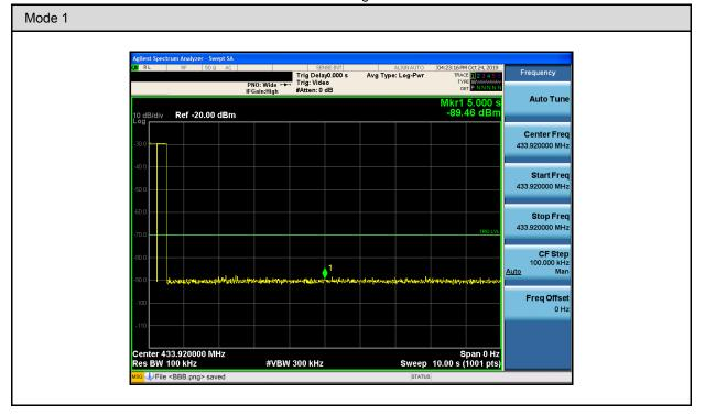
The EUT was complied with the requirement of FCC 15.231 (a) (1), which employed a switch that will automatically deactivate the transmitter within less than 5 seconds of being released.
