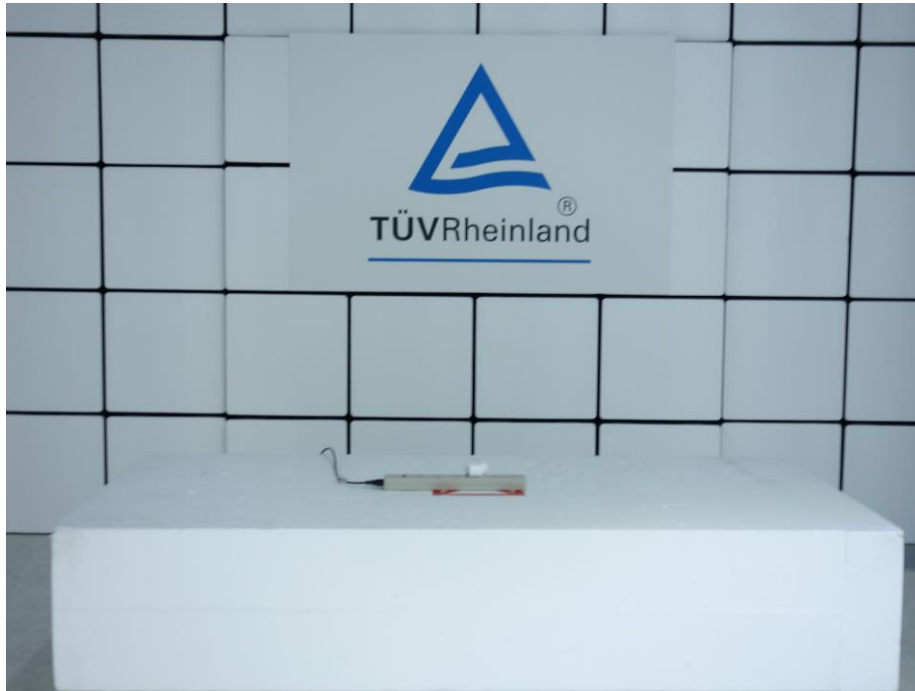
Photograph 1: Set-up for Spurious Emissions (Front View 1)
