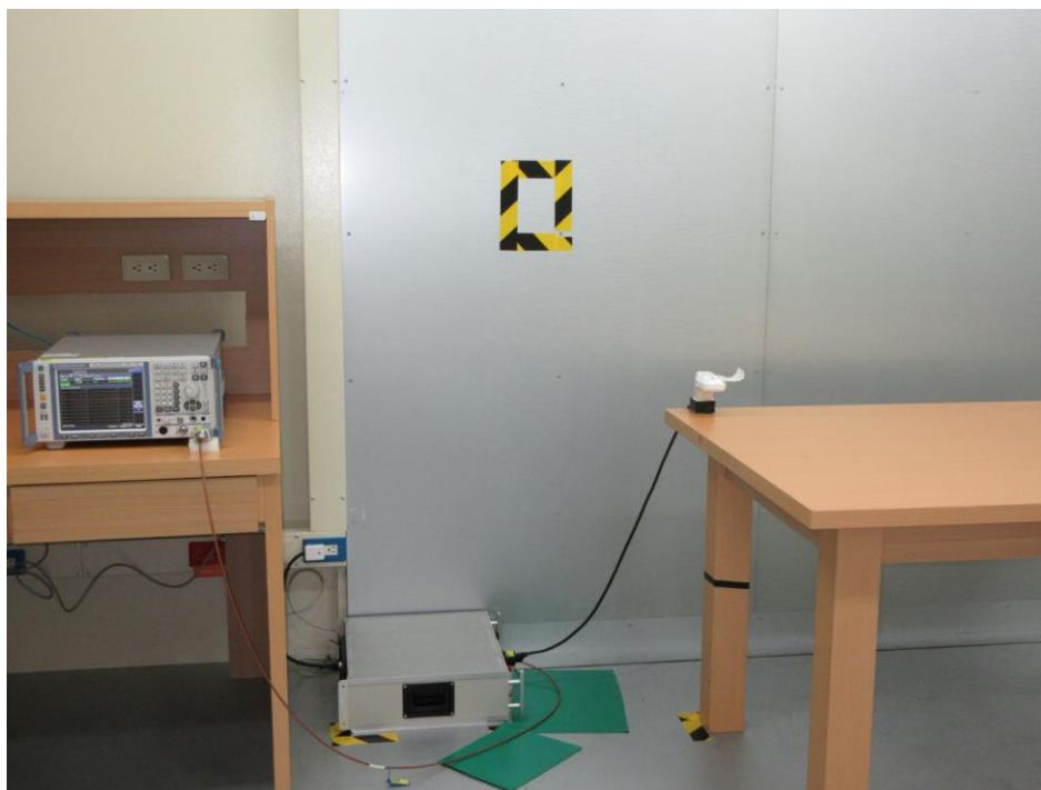
Photograph 6: Set-up for AC Mains (Front View)
