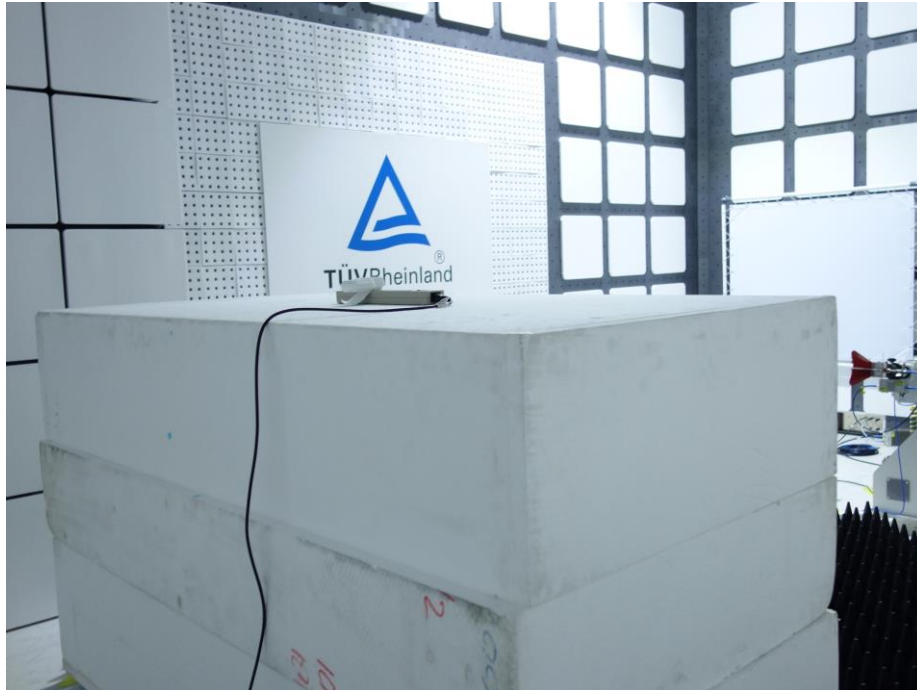
Photograph 5: Set-up for Spurious Emissions (Back View 3)
