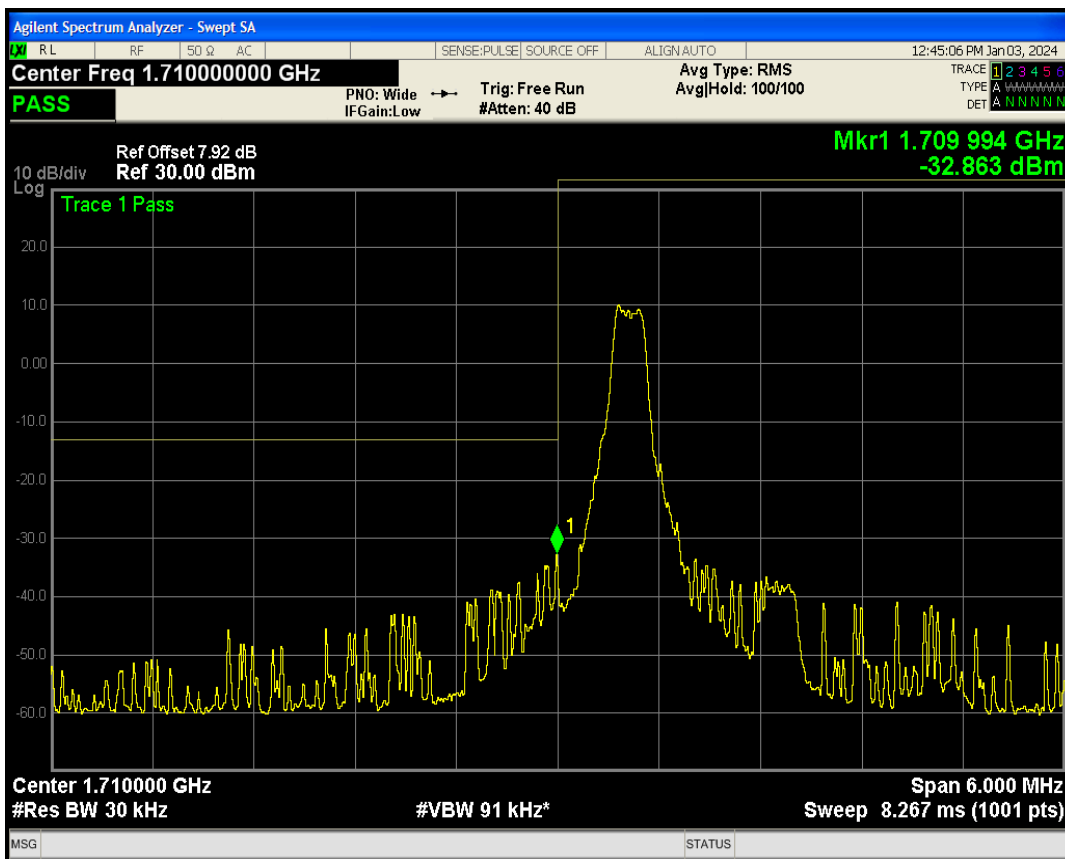
Band4 QPSK BW=3MHz Channel=19965 RB Size=6 Position=#0 NB Index=0
