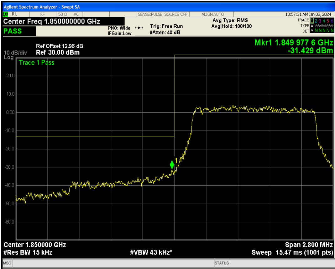
Band2 QAM16 BW=1.4MHz Channel=18607 RB Size=6 Position=#0 NB Index=0
