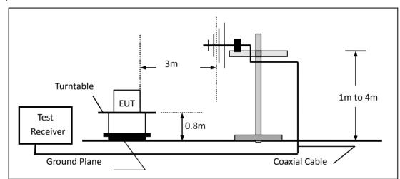
(c) For radiated emissions above 1000MHz
