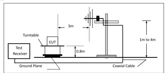
(c) For radiated emissions above 1000MHz
