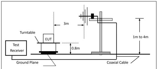
(c) For radiated emissions above 1000MHz
