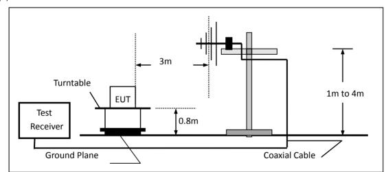
(c) For radiated emissions above 1000MHz
