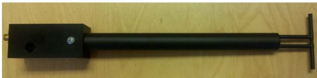
Figure 1 – MVG COMOSAR Validation Dipole
