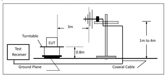
(c) For radiated emissions above 1000MHz
