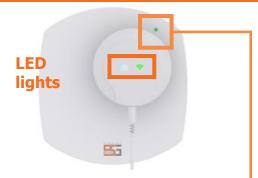
Plug the Echo 5G IDU into your wall outlet. Blue and green LED lights on the IDU will appear and blink before going solid. If the green light blinks for more than 30 seconds, consult the Troubleshooting Help on the back of this page.
