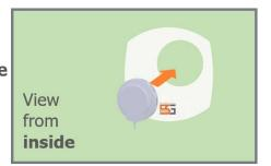
Remove the adhesive from the Velcro on the pre-attached spacer ring on the IDU and press to the glass in the circle of the alignment cling.
