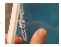
When you have loosened the adhesive enough you can carefully remove it by hand.
