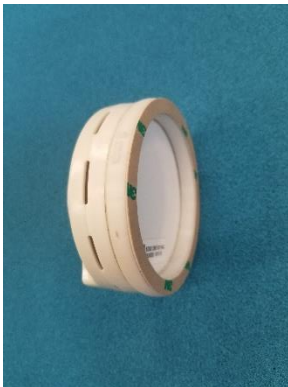
Assembled IDU, spacer ring, and Velcro-to-window adhesive
