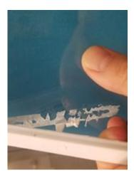
When you have loosened the adhesive enough you can carefully remove it by hand.
