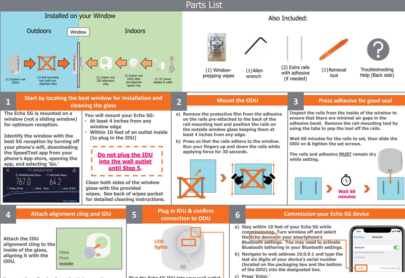
Remove the adhesive from the Velcro on the pre-attached spacer ring on the IDU and press to the glass in the circle of the alignment cling.
