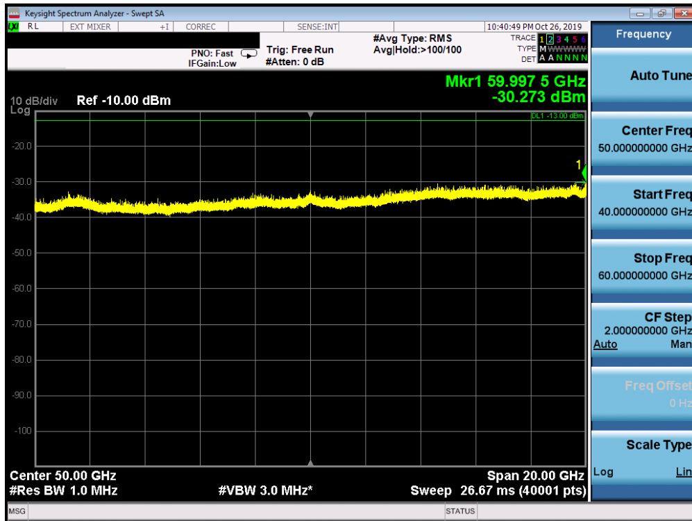
Plot 7-73. Patch Antenna Radiated Spurious Plot 40-60 GHz (1CC QPSK High Channel H Beam)
