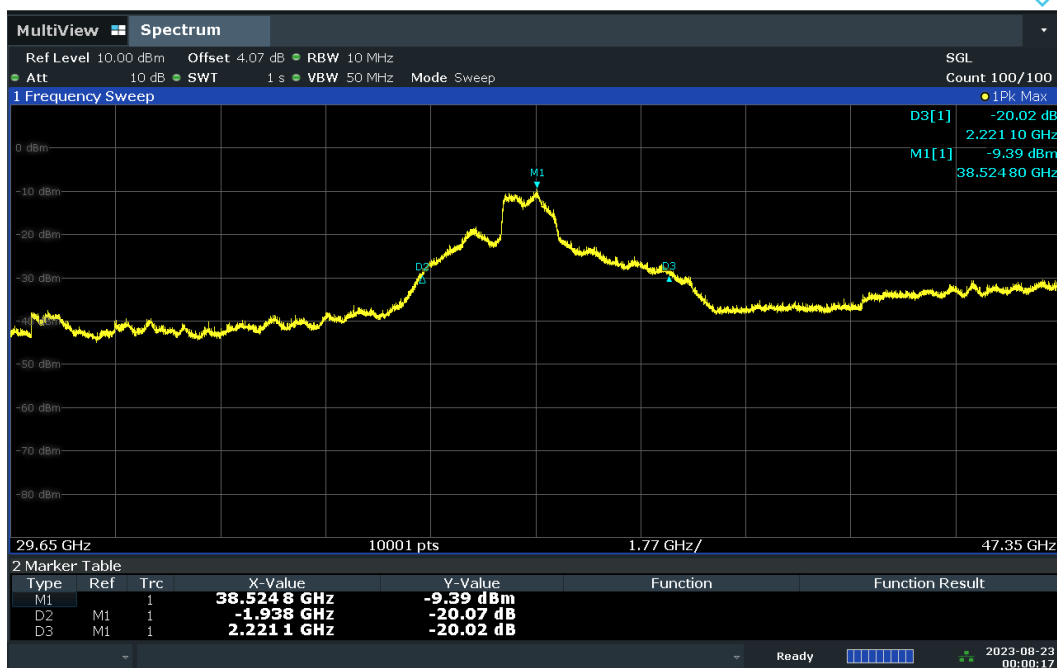
Plot 7-18. Out-Of-Band Rejection – H-DL Polarization
