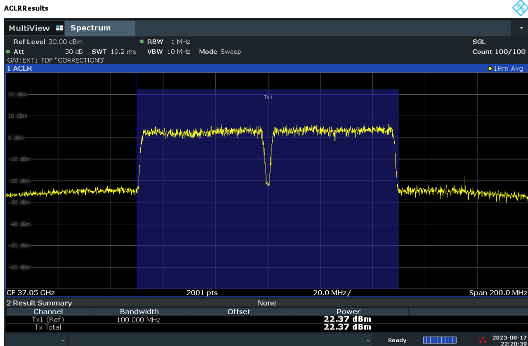
Plot 7-50. Conducted Power Plot – DFT-S – V-DL Polarization (50MHz-2CC – QPSK – Low Ch. – Full RB)
