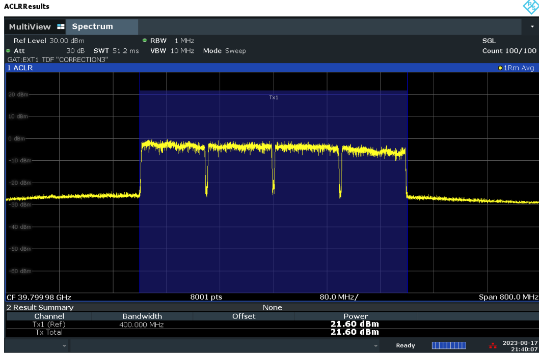
Plot 7-103. Conducted Power Plot – CP – V-DL Polarization (100MHz-4CC – QPSK – High Ch. – Full RB)
