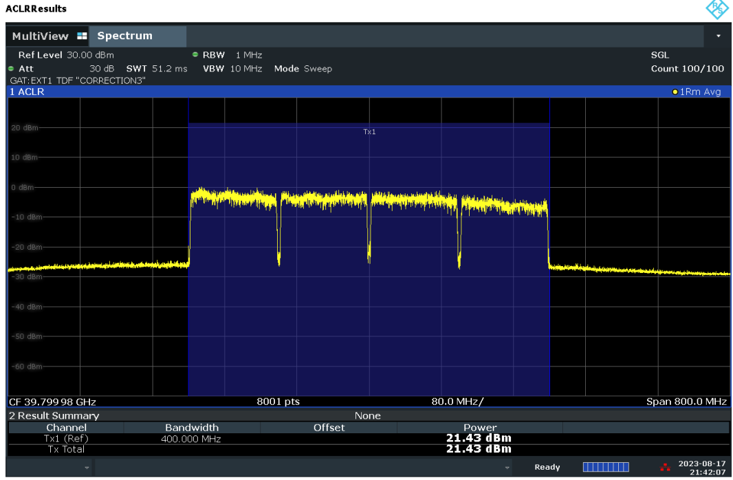
Plot 7-105. Conducted Power Plot – CP – V-DL Polarization (100MHz-4CC – 16QAM – High Ch. – Full RB)
