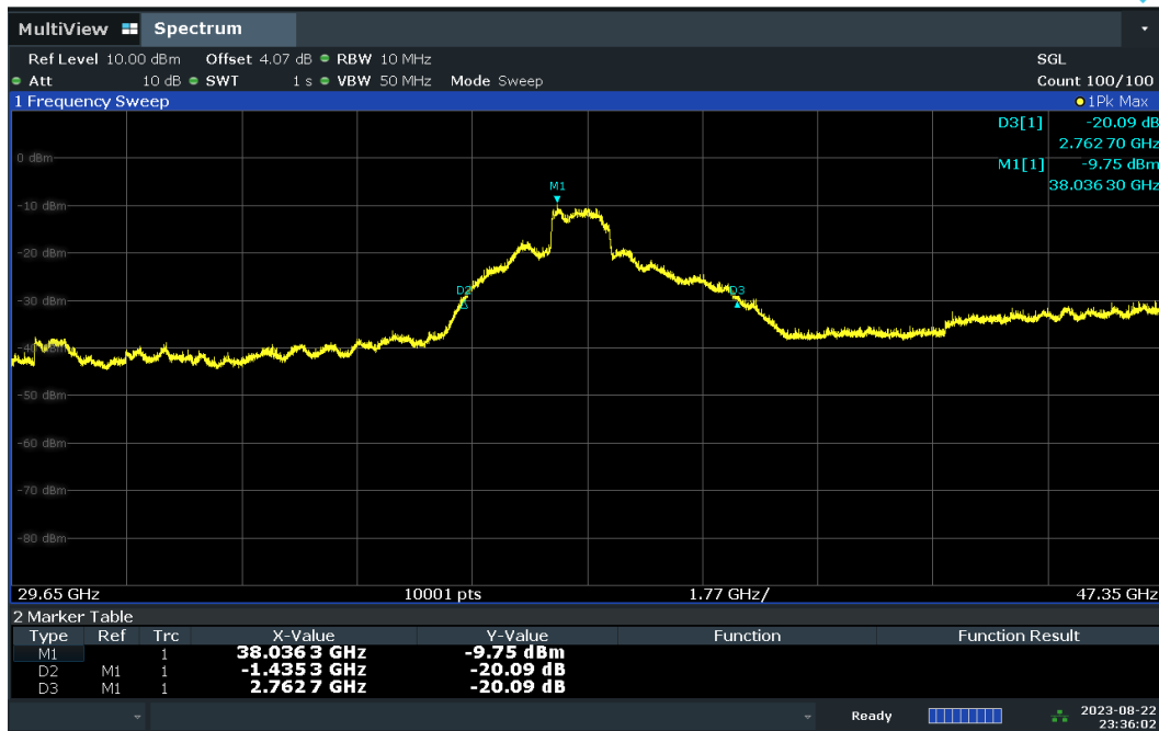
Plot 7-17. Out-Of-Band Rejection – V-DL Polarization
