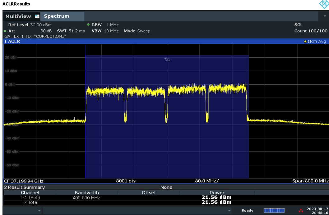
Plot 7-57. Conducted Power Plot – DFT-S – V-DL Polarization (100MHz-4CC – QPSK – Low Ch. – Full RB)
