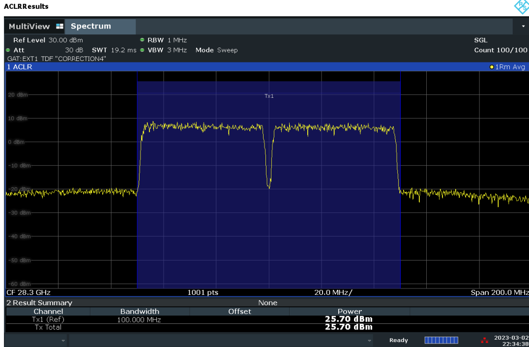
Plot 7-51. Conducted Power Plot – DFT-s – H-DL Polarization (50MHz-2CC – QPSK – High Ch. – Full RB)
