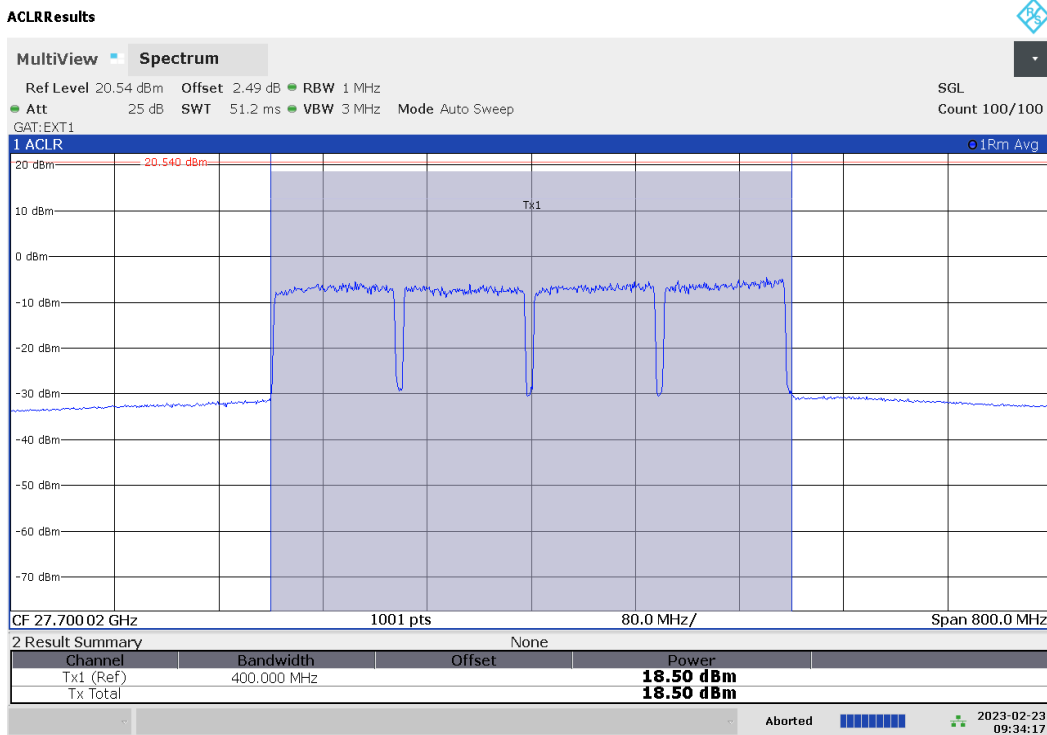
Plot 7-53. Conducted Power Plot – DU – V-UL Polarization (100MHz-4CC – QPSK – High Ch. – Full RB)
