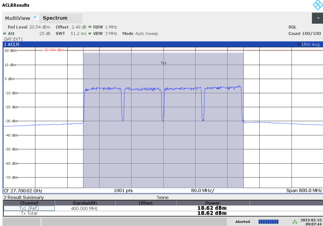
Plot 7-49. Conducted Power Plot – DU – V-UL Polarization (50MHz-1CC – 16QAM – Mid Ch. – Full RB)
