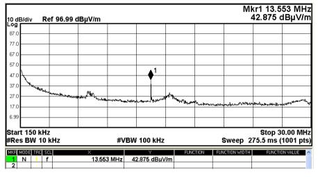
The peak value shown on the graph was 13.56MHz which the result was measured and calculated at page 7-8, others missions detected outside the spectrum mask are more than 20 dB below the FCC Limits
